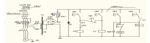
QS: Main switch QF: circuit breaker KM: Contactor TC: Transformer VC: ACDC converter FU: Fuse HL: Lamp SQ: Limit switch SB1: UP button SB2: Down button YV1: Hydraulic valve YV2: Pneumatic valve BZR: Buzzer KT: Timer SB3: Lock button
