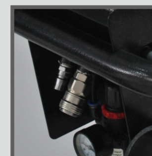
Air inlet and air outlet for pneumatic tools
