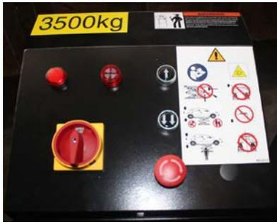
3. Levelling two platform (When operate lift, two platforms un-levelling)
