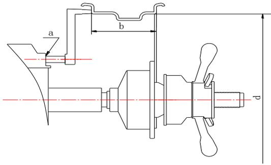
Move gauge to touch edge of rim (Fig.1), read the value of distance, press **a+** and **a-** to change, set “a” value.
