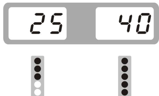
4.1.7. Anticlockwise moving wheel slowly, the displays with left LED's lit up full indicate the correct angular position where to mount the counterweights (12 o'clock position) inside, as Fig.4, clip the counterweight.
